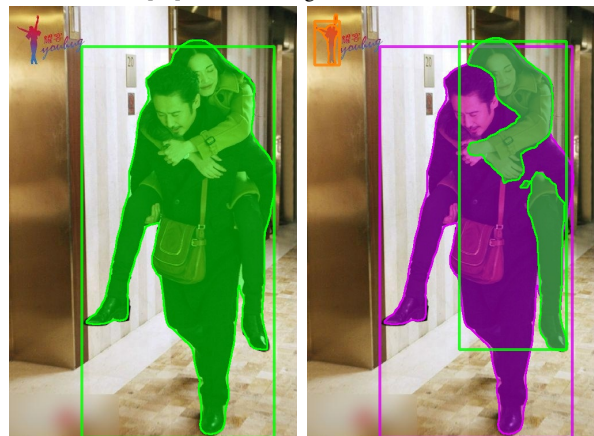
(b) Two instances in one detection are resolved by refining segmentation masks with SAM [21] prompted by the detected pose. Left – RTMDet [18], right – BMP. Note that the detection of the woman is improved, but the right leg is still wrong.
