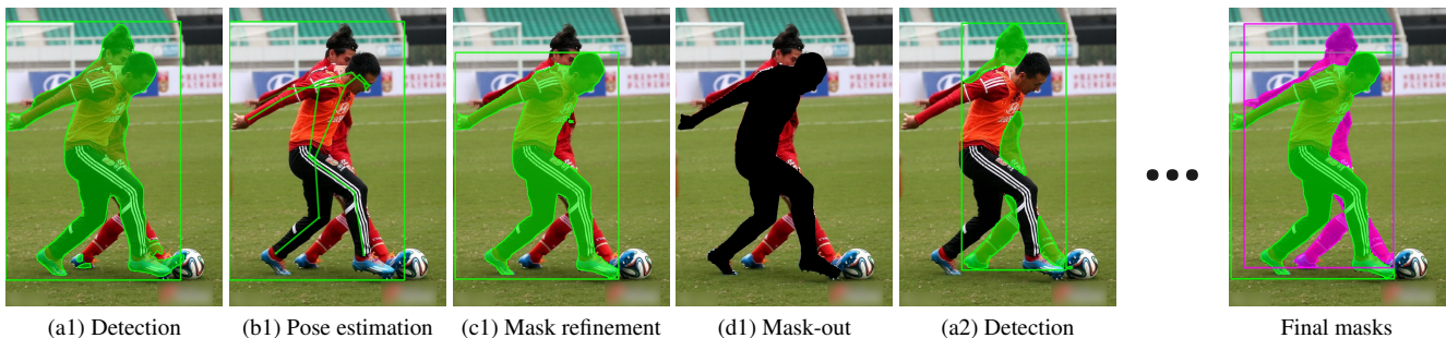
Figure 1. The BBox-Mask-Pose (BMP) method. Steps (a) – (d) repeat until no new detections in step (a) are found. The loop can start from a bounding box (a.), pose (b.), or segmentation mask (c.). In this example, the background player is first undetected in step (a1). BMP correctly fits the foreground player’s pose (b1) and corrects his segmentation (c1). After masking the foreground player (d1) the background player is detected (a2) and his body segmented (final masks).
